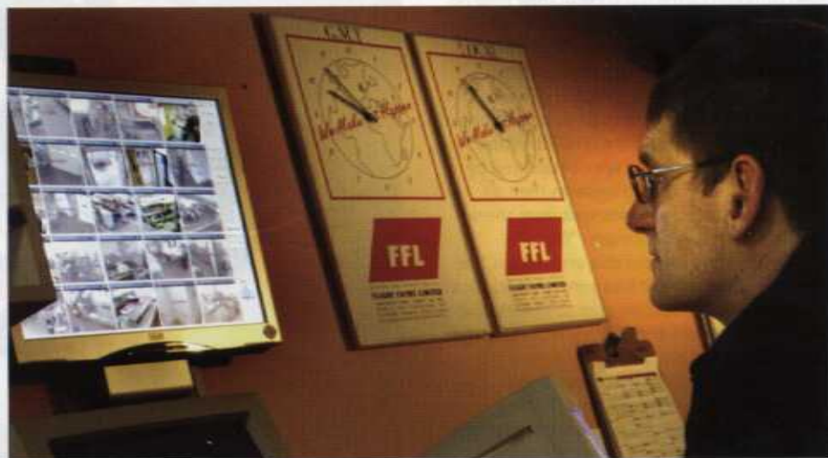
Inside the Operations Room. A single 19-inch flat panel display monitor mounted on the wall enables staff to monitor high resolution images from all cameras on the site.
